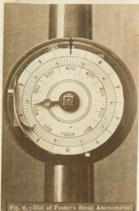
Fig. 6.—Dial of Foster's Small Anemometer.
