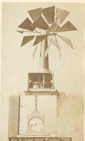
Fig. 8.—Long Shaft Windmill Vane.
