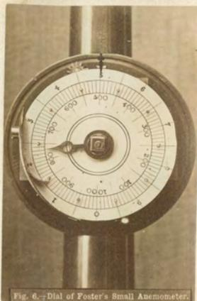
Fig. 6.—Dial of Foster's Small Anemometer.
