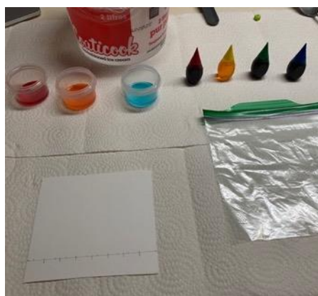
Figure 4: Whatman #1 chromatography paper with divisions for spotting
