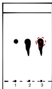
Figure 2: Tailing effect of samples - lanes: (1) well resolved spot, (2) spot with tailing, (3) determining the center of migration for a spot with tailing.
