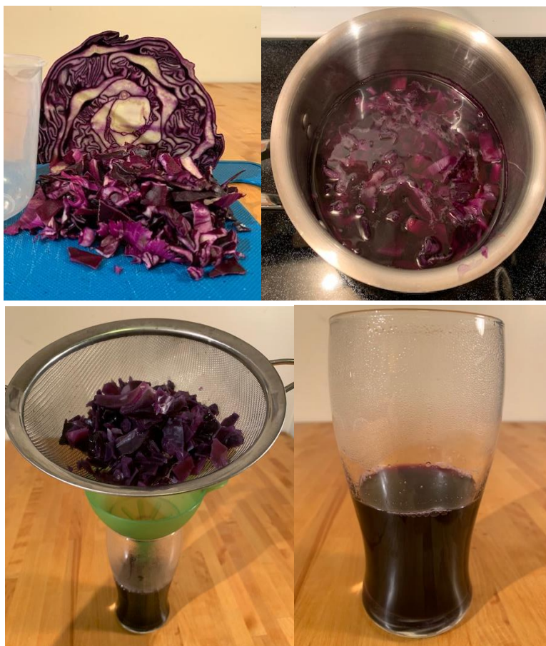
Figure 3: Cutting, boiling and filtering the red cabbage leaves to recuperate the homemade acid-base indicator.
