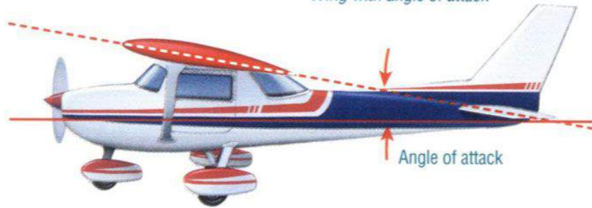
Figure 4-24 Wing with angle of attack
